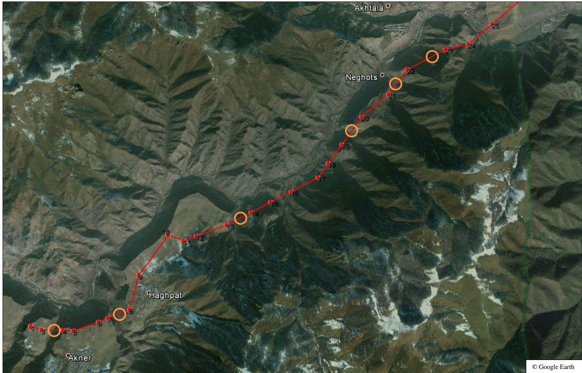
Map 9-1: Line sections of planned 110 kV Lalvar and Noyemberyan OTLs crossing gorges, where bird diverters shall be installed (orange circles) - south-western part
